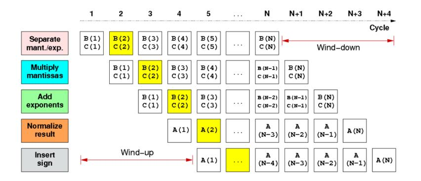
First result is available after 5 cycles (=latency of pipeline)! Wind-up/-down phases: Empty pipeline stages
